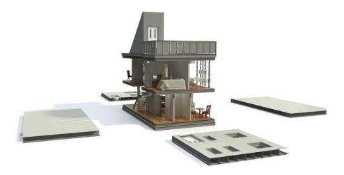
Startlink is a pultruded component kit which can be rapidly assembled into a variety of low-rise building forms without metal fastenings.
