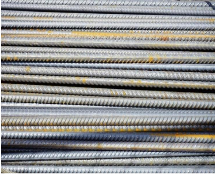
Steel rebar is readily available and widely used in building and construction applications, but it is susceptible to corrosion. (Image courtesy of Hans Braxmeier/Pixabay.)
